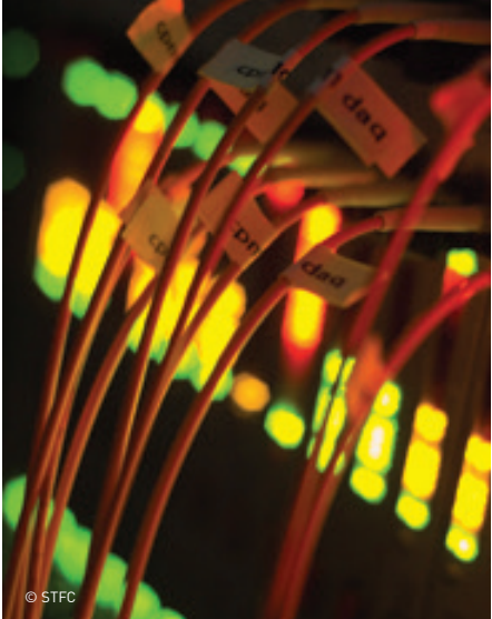
Optical Links going to the Readout Module of the ATLAS Readout System
