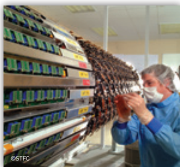
Construction of the barrel section of the ATLAS SCT
